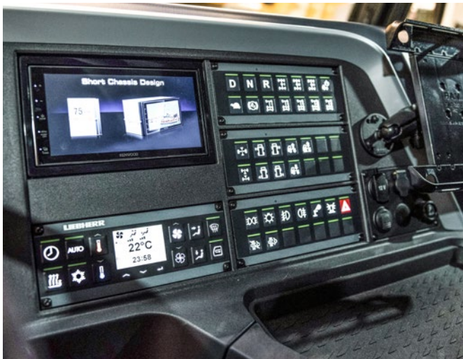
Modern automatic heating and air conditioning system and self-explanatory button modules
