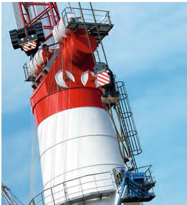
Truly heavy – giant shackles and steel ropes as thick as an arm are used to secure the top section of the boom.
