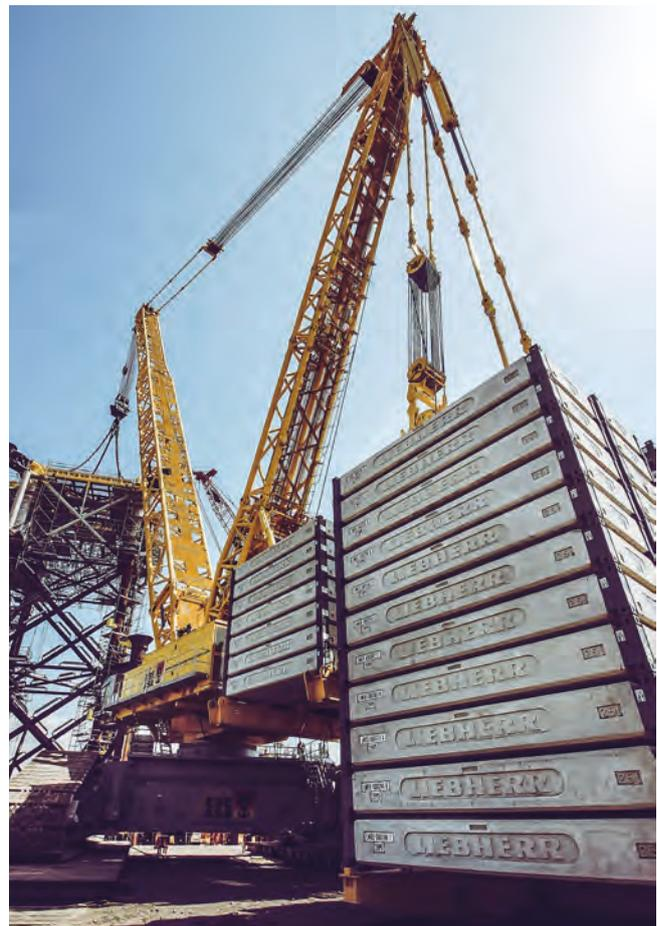
For low cost transport, the ballast slabs for the LR 13000 have precisely the same dimensions as a 20 foot container and can be loaded with a spreader.
