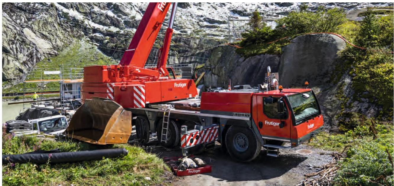
The VarioBase® variable support base makes it possible to use the crane.
