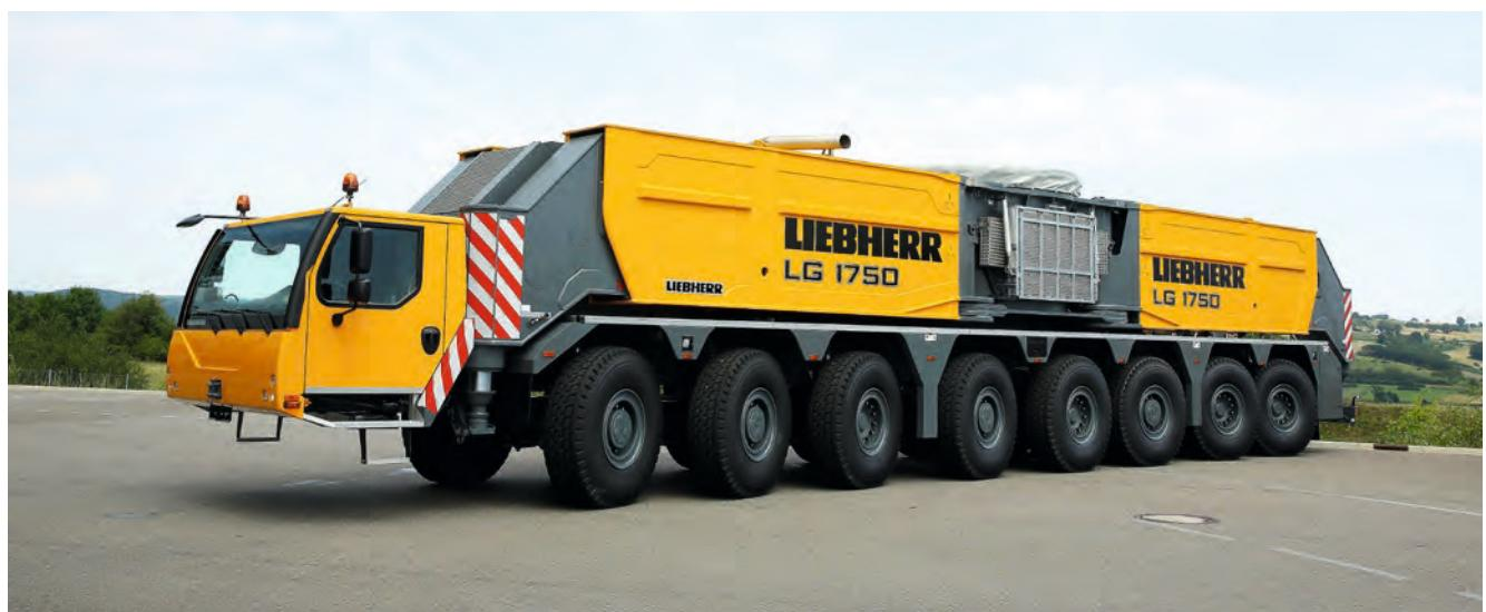
The special success of the LG 1750 is certainly also due to the fact that we did something new with this crane. We did not use an existing chassis from a telescopic crane, as we had done in the past, but designed a very specific new undercarriage. The focus of this process was to enable the crane to travel between sites with some of its equipment at low cost. That is why it has particularly strong crane axles and tyres. This means that the LG 1750 can carry up to 40 tonnes per axle.
