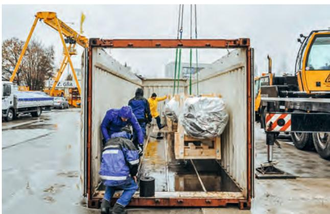
Within three days, the LTM 1040-2.1 mobile crane was disassembled into individual parts for transport. Each part could not exceed the weight limit of eight tonnes.
