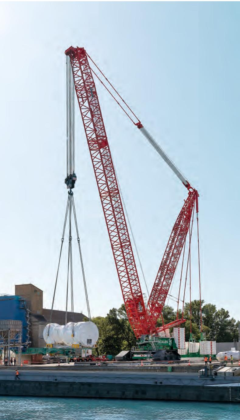
A gas turbine can weigh up to 450 t – which is why the LR 11000 has been permanently installed at the port.
