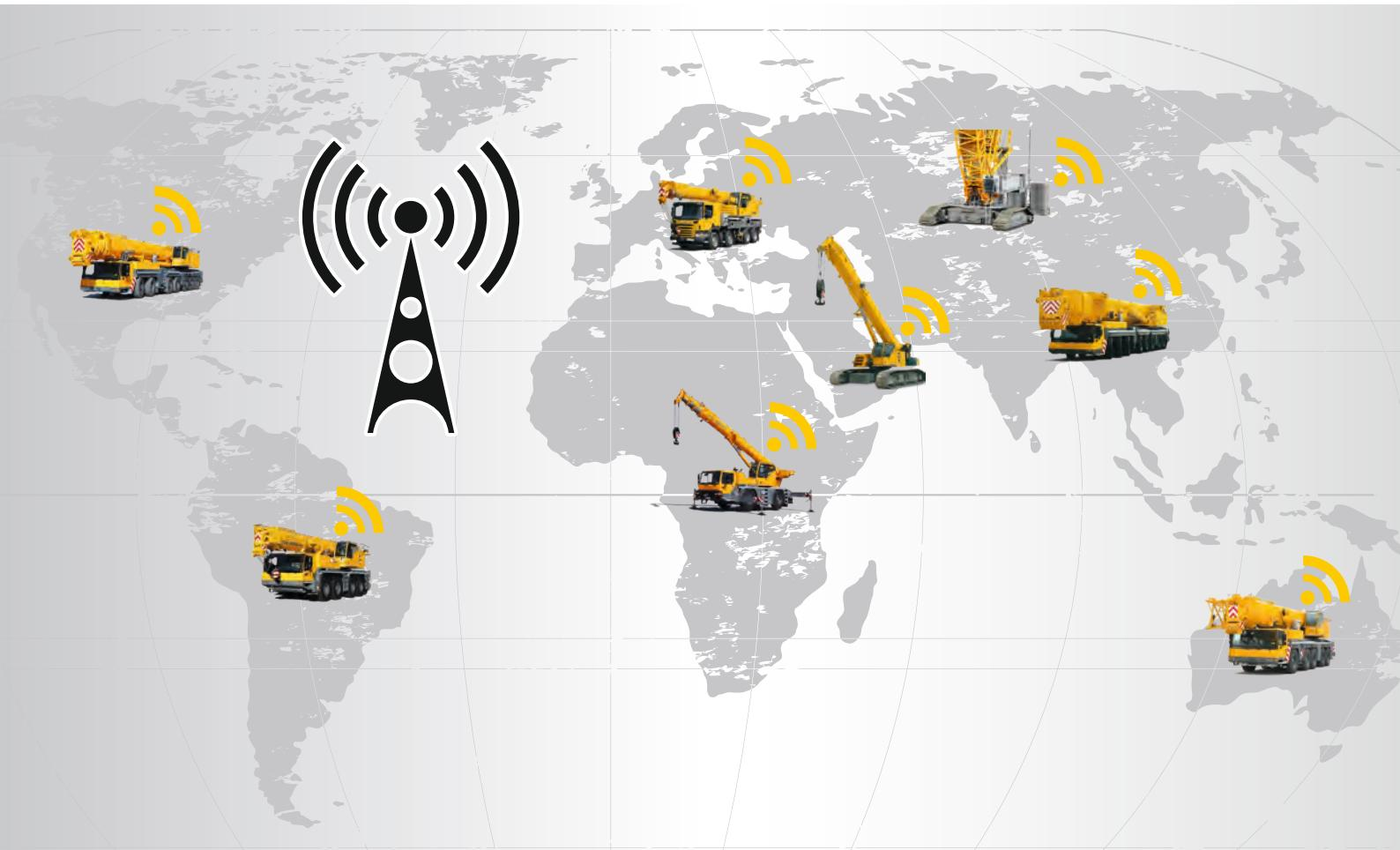
For many years we used GSM technology for remote diagnostic purposes as it was state of the art. However, in many countries it performed poorly or not at all. We therefore decided to improve the system. Data transfer is now possible throughout the world using an encrypted 3G connection. The new system is already fitted on many models in the current crane range.
