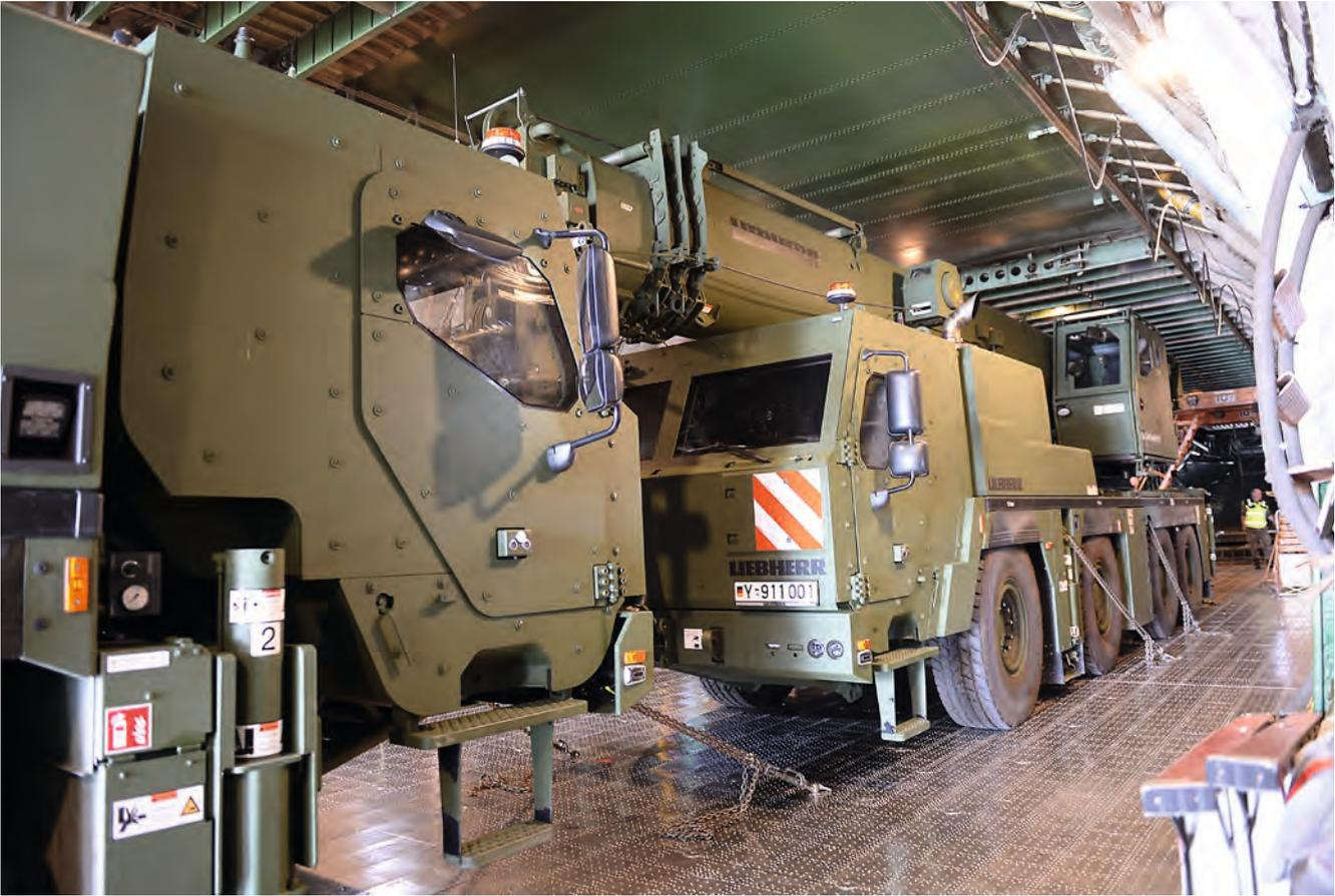
The first are already attached – each crane is secured in the Antonov by 36 chains.
