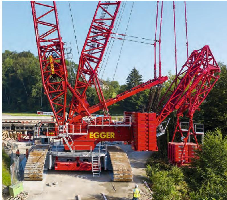
The benefit of the VarioTray – with the central section of the ballast disconnected from the derrick boom, the crawler crane can position its suspended ballast pallet itself.
