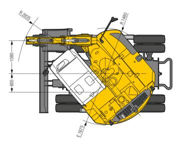
**Min. turning radius on tyres 9.00-20** Four wheel steering 4,29 m
