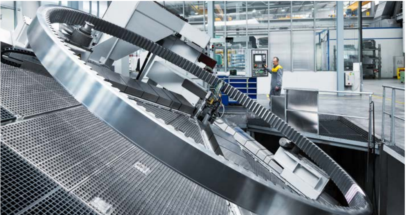
Inductive hardening of tooth flanks of large diameter bearings
