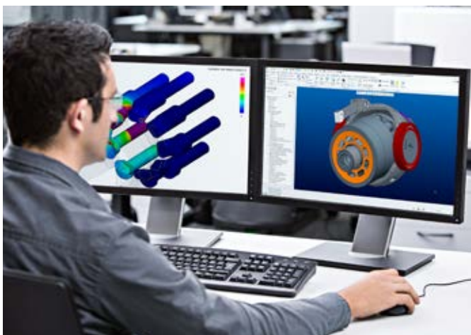
Development of axial piston unit with use of the finite element method (FEM)
