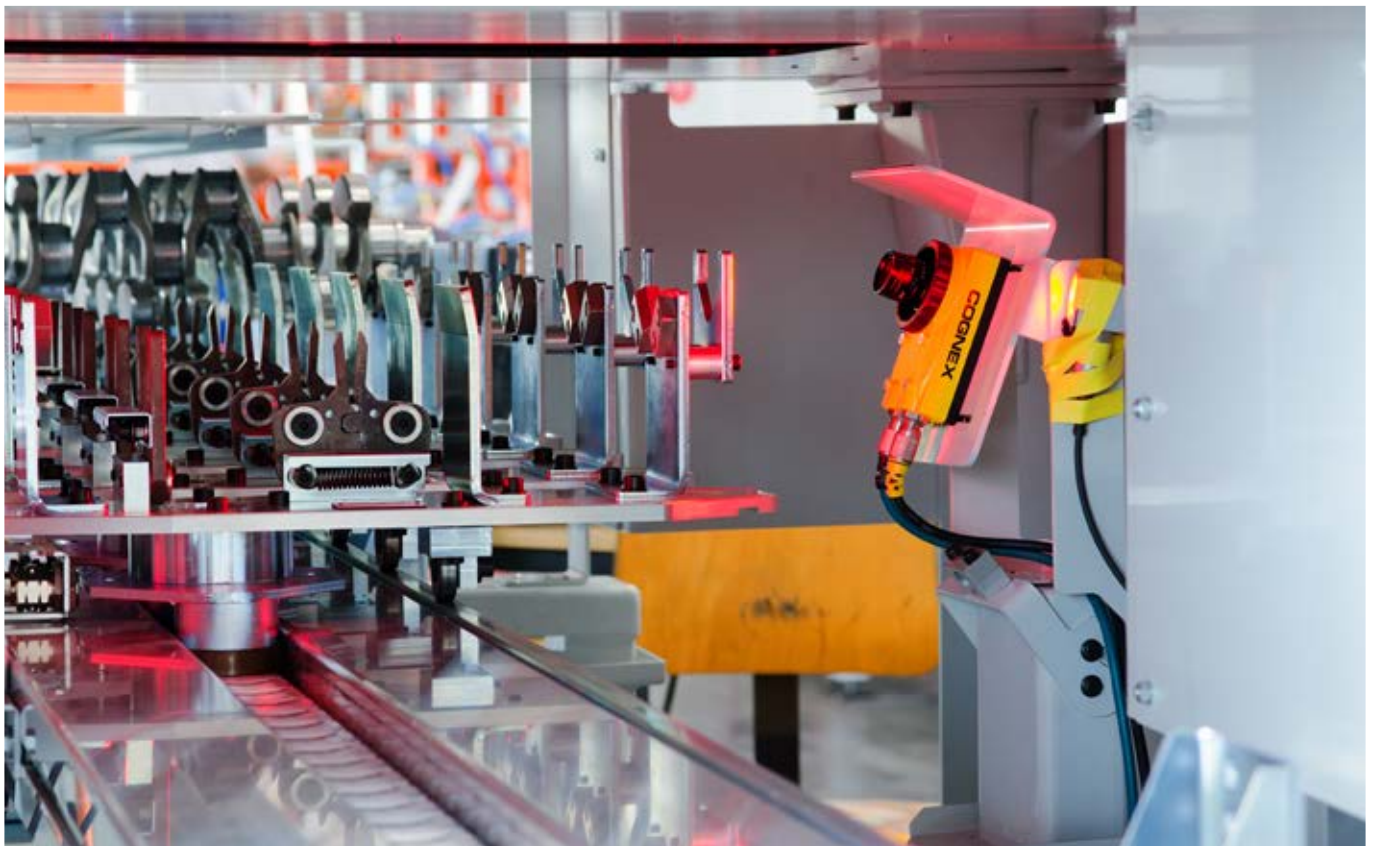
The plastic chain conveyor (KKB) as conveying system for crankshafts for example
