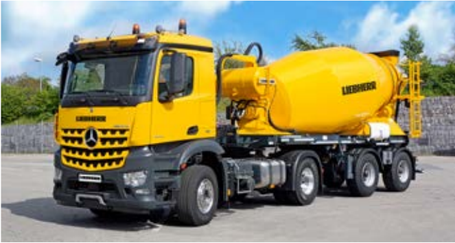
The truck mixer HTM 1004 ZA/38 is approved for a total weight of 38 t
