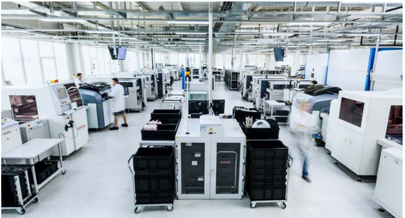
Fitting circuit boards with SMD technology
