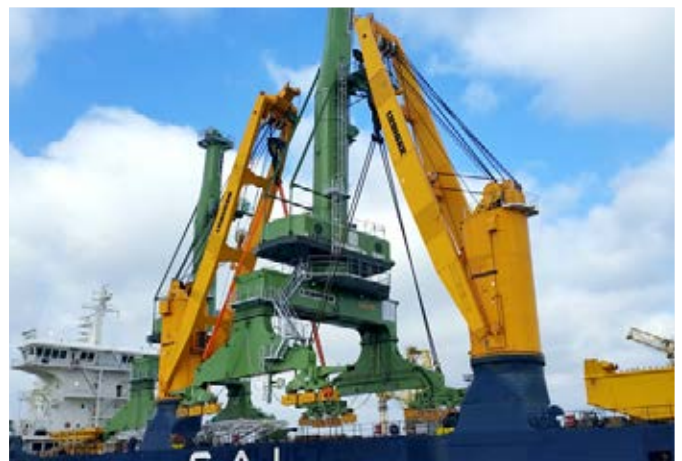
Two CBB 4700 ship cranes in tandem lift during the transfer of a Liebherr LPS in Rostock
