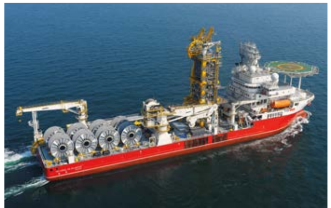
Pipe Laying Service Vessel (PLSV) with a RL-K 7500 for pipe installation in deep waters
