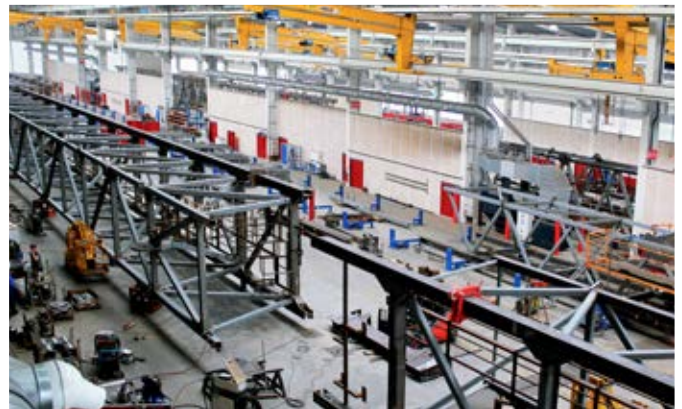
Assembly of a ship to shore container crane boom in the Liebherr factory in Killarney (Ireland)
