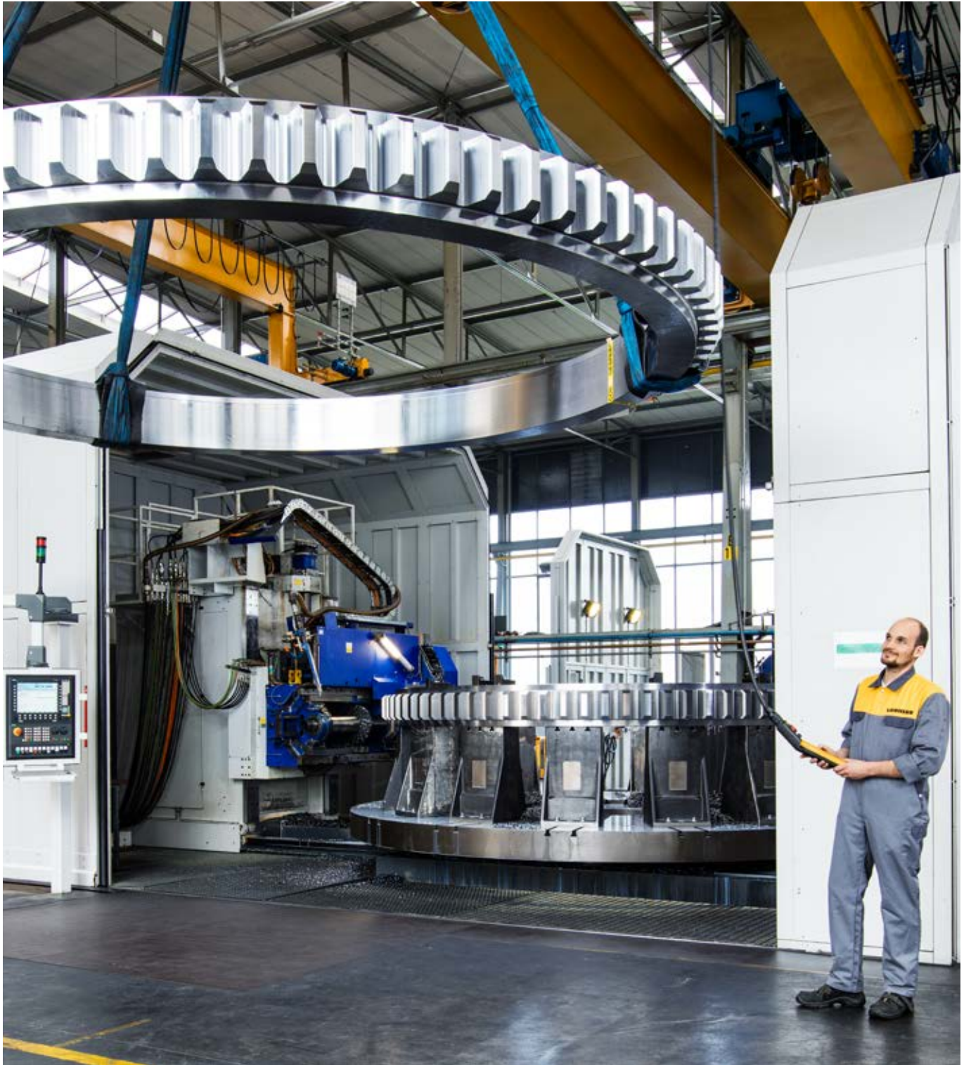
Liebherr gear cutting machines for soft and hard machining of cylindrical gearing with workpiece diameters between 60 mm and 16,000 mm
