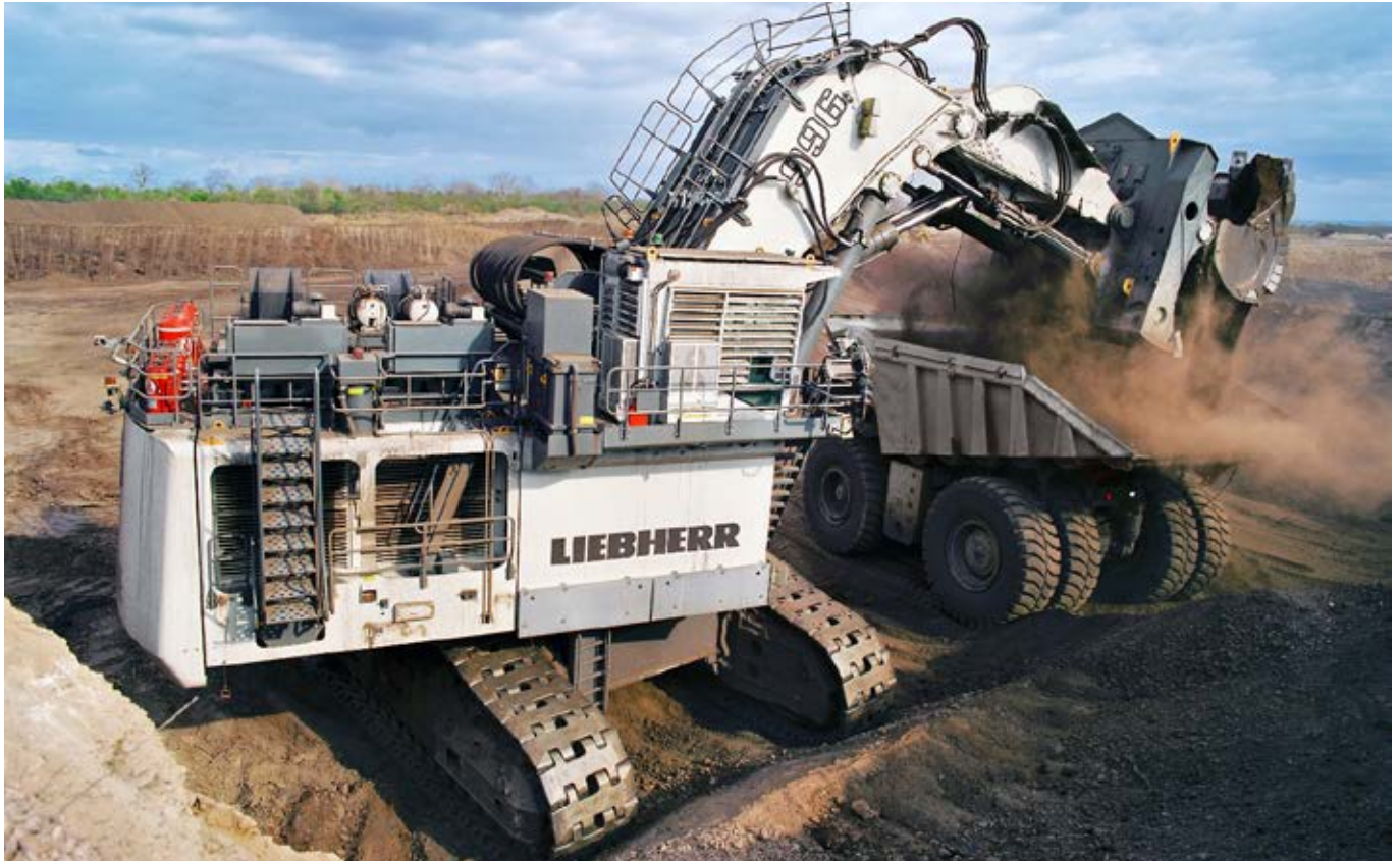
The Liebherr R 996 B with face shovel configuration in South Africa
