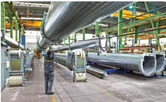
Assembly of telescopic booms
