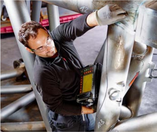
Ultrasonic testing of weld seams
