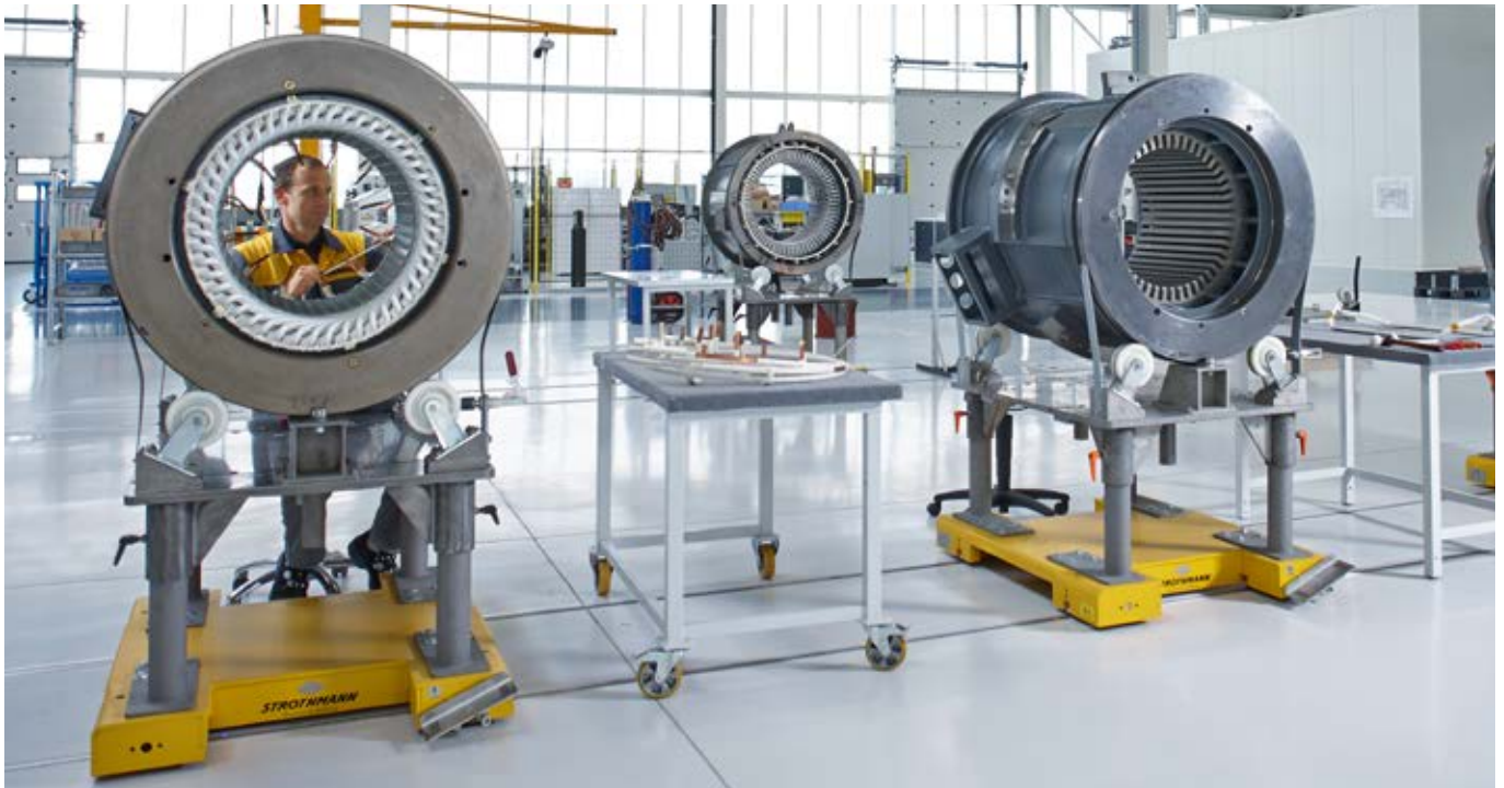
Winding room of electrical machines for mining trucks and port cranes
