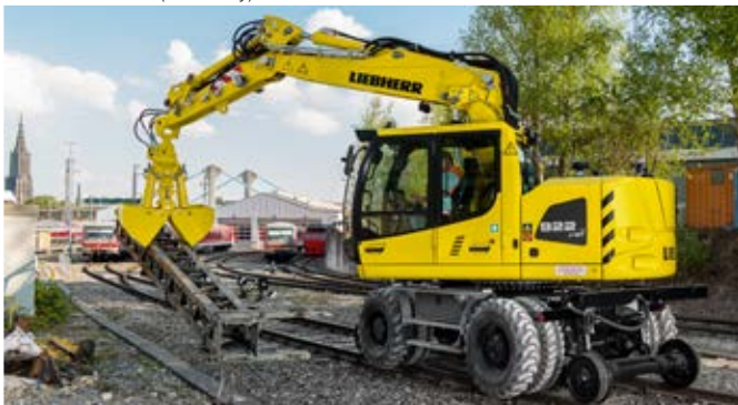
The A 922 Rail Litronic in use for load lifting in the area of Ulm central train station (Germany)
