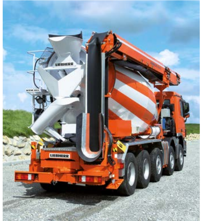
The truck mixer HTM 1004 with double telescopic conveyor LTB 12+4+1
