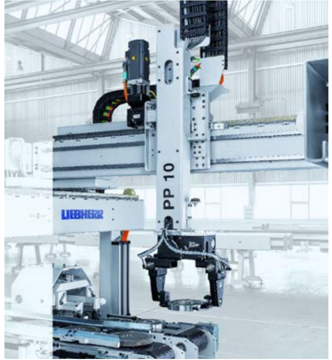
Portal robot for workpieces with weight between 0.5 kg to 1,500 kg
