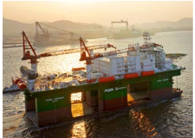
BOS cranes on a semi-submersible accommodation vessel lift loads up to 300 tonnes
